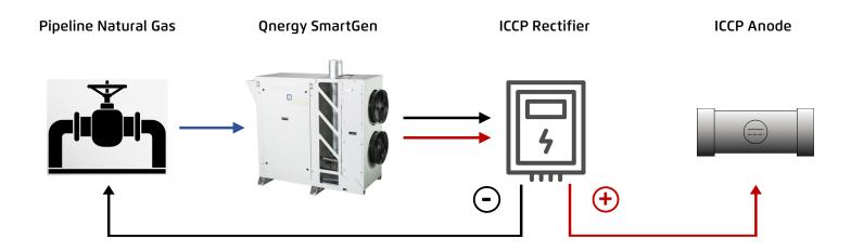
The Smartgen configured to ICCP Application is one of 5 standard configurations to meet your remote power needs.
